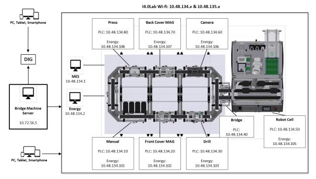
Architecture of Industry 4.0 lab base ICT system (focus on Levels 0, 1, 2 of Enterprise-control system ref. (IEC) 62264:2003)
